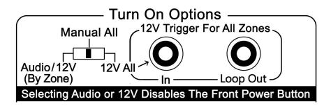
The setting of the rear panel Turn On Options Switch determines whether all six zones turn on and off together or if each zone turns on and off individually. *There are three positions for this switch:*
